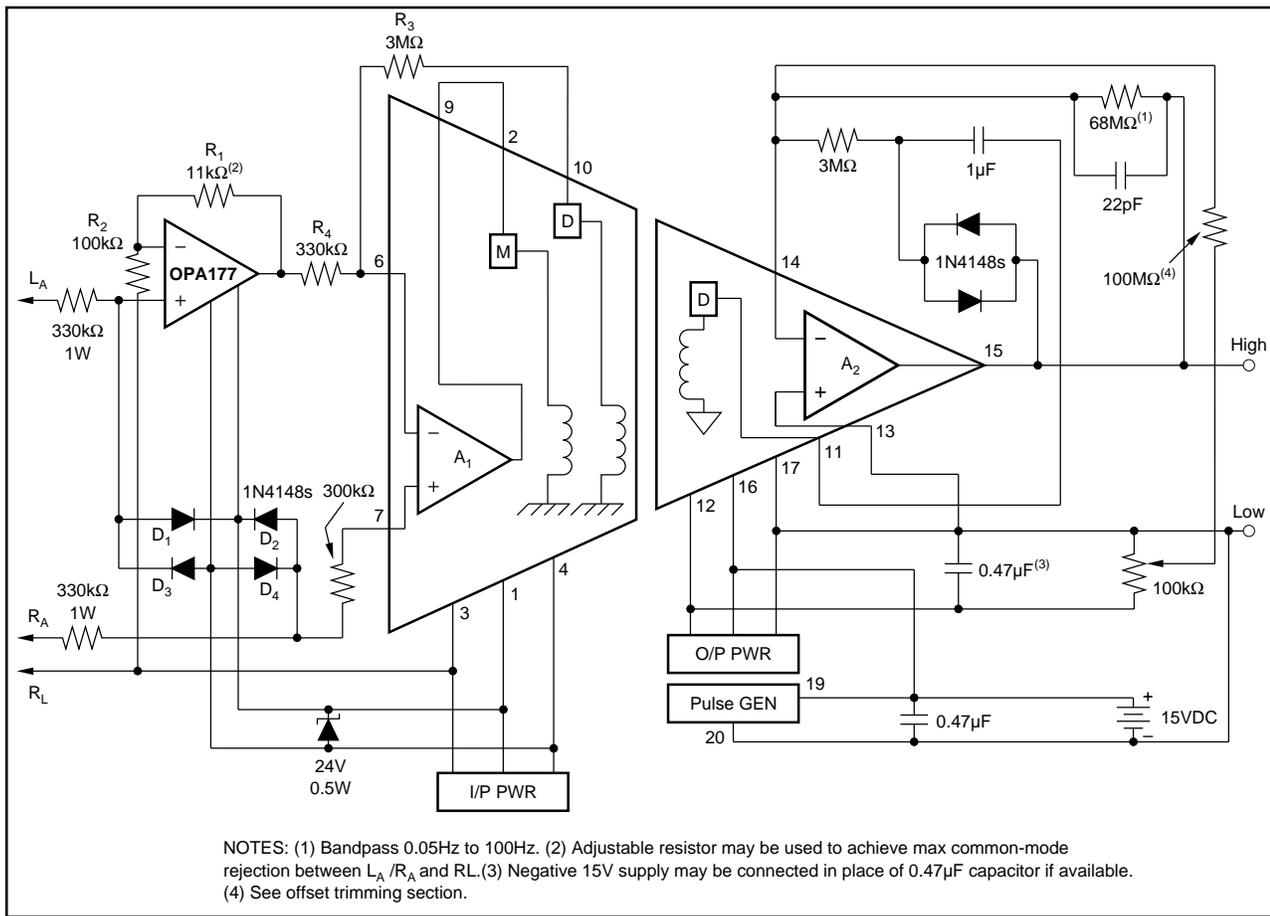
FIGURE 6. ECG Amplifier.
