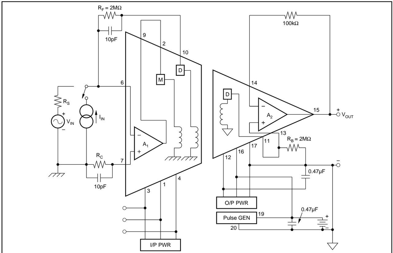
FIGURE 4. Power: Two-Port, Single Supply; Signal: Inverting Gains.
