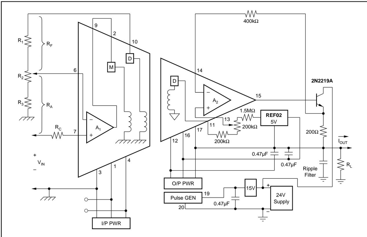
FIGURE 10. Isolated 4mA to 20mA  $I_{OUT}$ .
