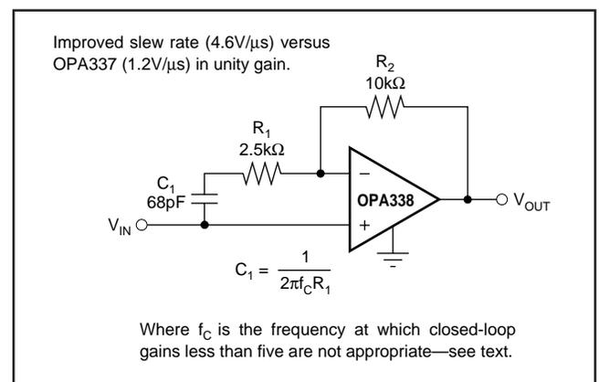
FIGURE 3. Compensation of OPA338 for Unity-Gain Buffer.
