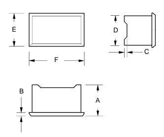
**Panel Cutouts**: See the Mechanical Specifications section of the DMS-20PC (data sheet number DS-0271) or DMS-30PC (data sheet number DS-0258) Series product data sheets for detailed panel cutout and panel mounting dimensions.
