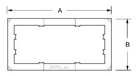
**Description:** Part numbers 39-2165110 (for all DMS-30/40 meters) and 39-2165105 (for all DMS-20 meters) metal retaining clips can be used as spares for damaged or lost clips and for securing blank cases to panels.
