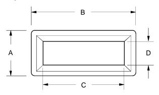
**Description:** DATEL part numbers 39-2359620 (for DMS-30PC and DMS-40PC red LED meters) and 39-2359621 (for DMS-20PC red LED meters) can be used when DMS meters are mounted on a pc-board which is situated behind a panel. Both bezels are made of black ABS plastic and easily snap into appropriately-sized cutouts (see chart for cutout dimensions) in metal panels whose thickness is between 0.040"(1.0mm) and 0.125"(3.2mm).
