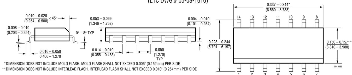
\*DIMENSION DOES NOT INCLUDE MOLD FLASH. MOLD FLASH SHALL NOT EXCEED 0.006" (0.152mm) PER SIDE
