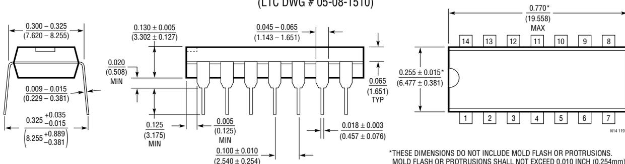
\*THESE DIMENSIONS DO NOT INCLUDE MOLD FLASH OR PROTRUSIONS.
