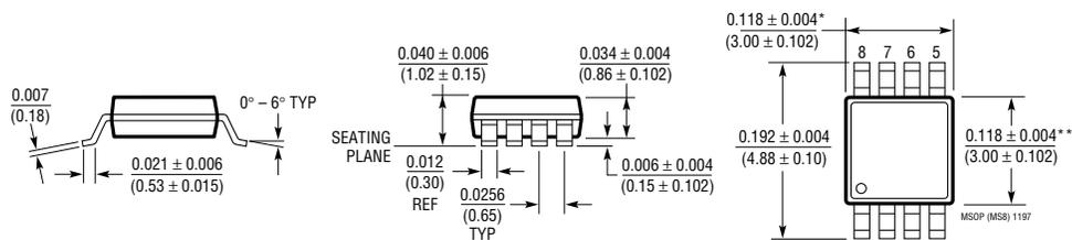
\* DIMENSION DOES NOT INCLUDE MOLD FLASH, PROTRUSIONS OR GATE BURRS. MOLD FLASH, PROTRUSIONS OR GATE BURRS SHALL NOT EXCEED 0.006" (0.152mm) PER SIDE
