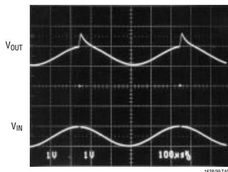
Figure 2. Lowpass Slope Limiting Filter with OTC
