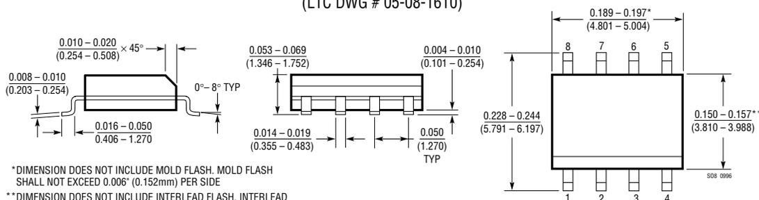
\*DIMENSION DOES NOT INCLUDE MOLD FLASH. MOLD FLASH SHALL NOT EXCEED 0.006" (0.152mm) PER SIDE
