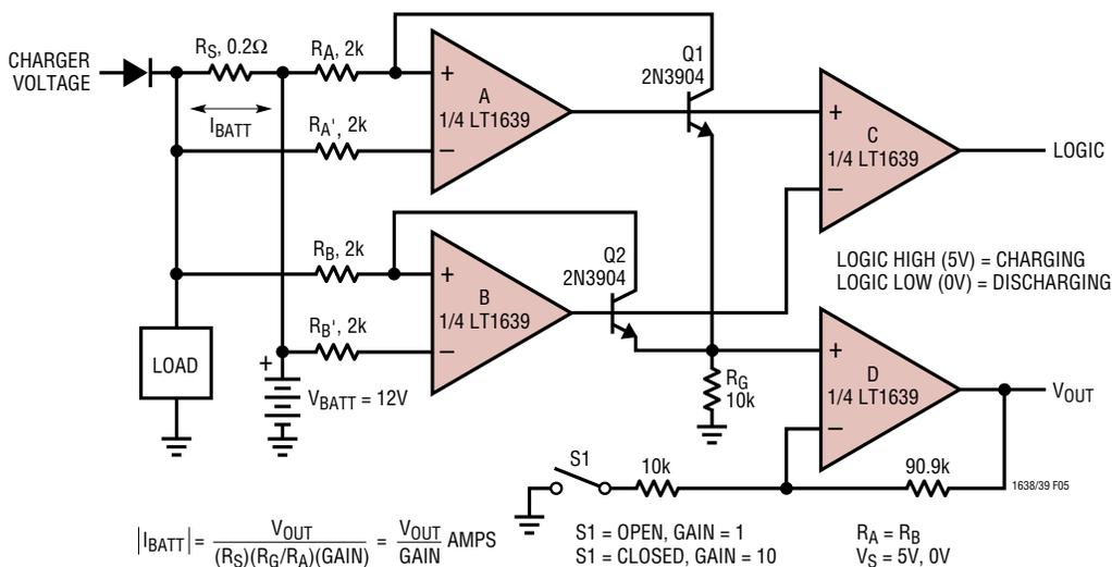
Figure 5. Battery Monitor
