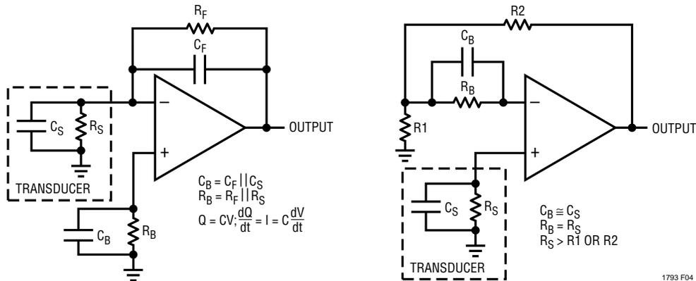
**Figure 4. Inverting and Noninverting Gain Configurations**
