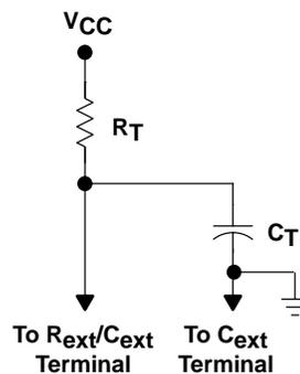
Figure 2. Timing-Component Connections
