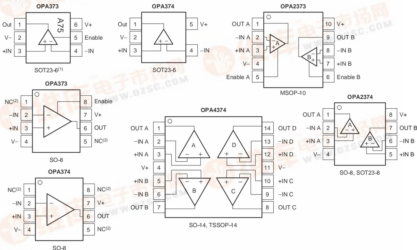
(1) Pin 1 of the SOT23-6 is determined by orienting the package marking as shown.
