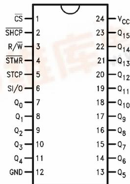
74F673A 16-Bit Serial-In, Serial/Parallel-Out Shift Register
