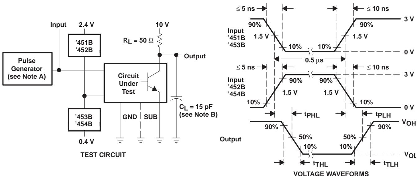
NOTES: A. The pulse generator has the following characteristics:  $PRR \leq 1\text{ MHz}$ ,  $Z_0 = 50\ \Omega$ .
