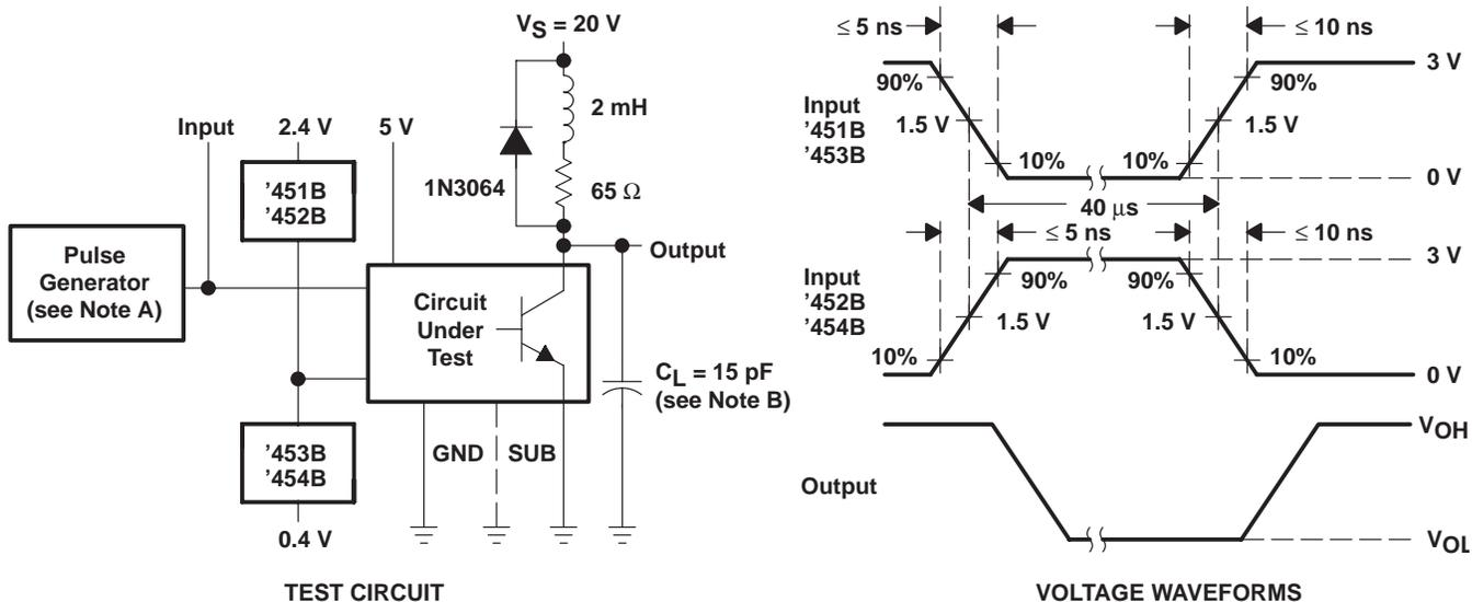
NOTES: A. The pulse generator has the following characteristics:  $PRR \leq 12.5\text{ kHz}$ ,  $Z_0 = 50\ \Omega$ .
