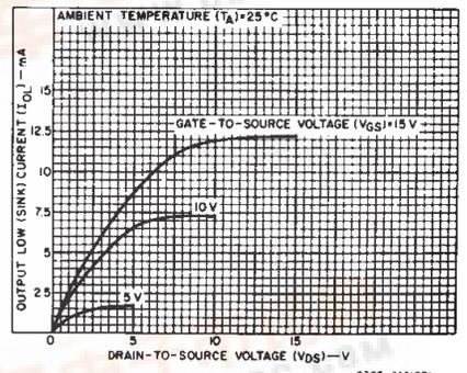
Fig. 2 — Minimum output low (sink) current characteristics.
