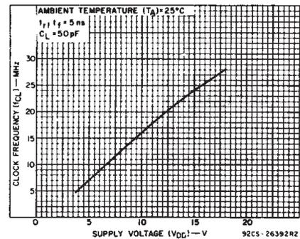
Fig. 8 — Typical maximum clock frequency vs. supply voltage.
