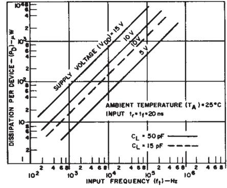
Fig. 9 – Typical power dissipation vs. frequency.
