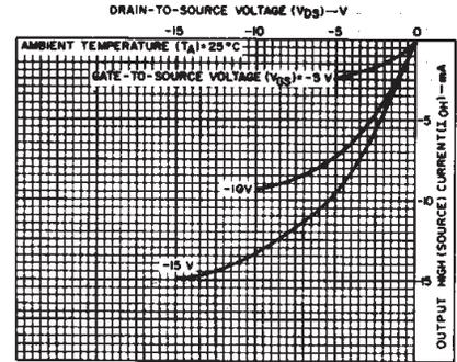
Fig. 4 — Minimum output high (source) current characteristics.
