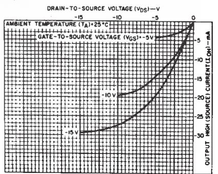
Fig. 3 — Typical output high (source) current characteristics.
