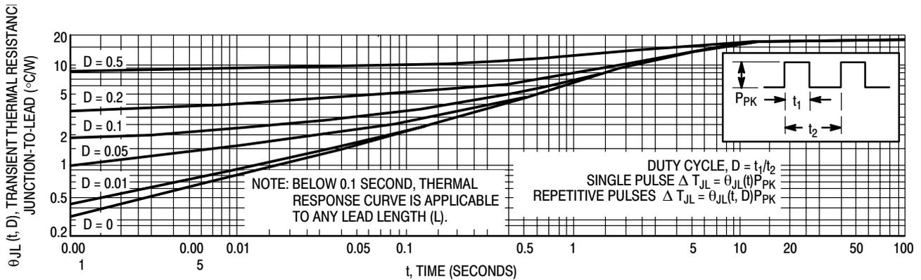
**Figure 4. Typical Thermal Response**
