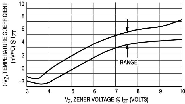
Figure 2. Temperature Coefficient-Range for Units 3 to 10 Volts
