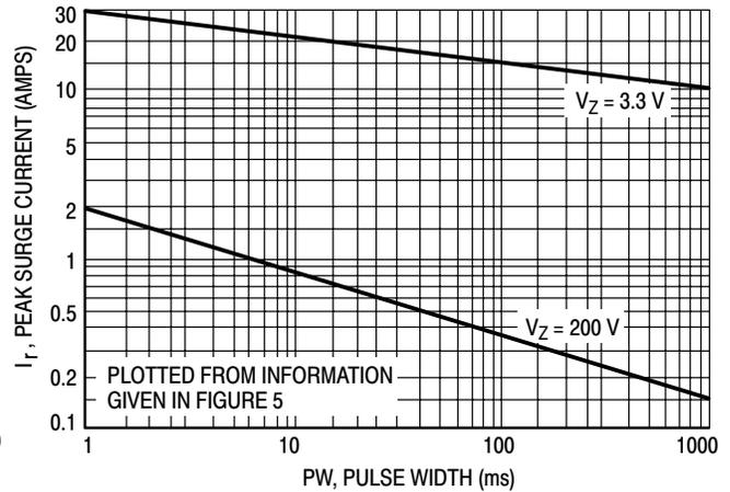
**Figure 6. Peak Surge Current versus Pulse Width**
