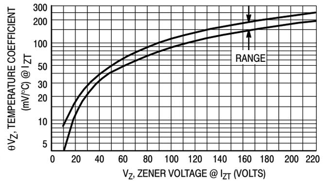
Figure 3. Temperature Coefficient-Range for Units 10 to 220 Volts
