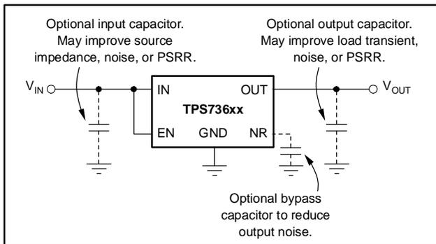
**Figure 31. Typical Application Circuit for Fixed-Voltage Versions**
