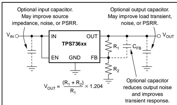
**Figure 32. Typical Application Circuit for Adjustable-Voltage Versions**
