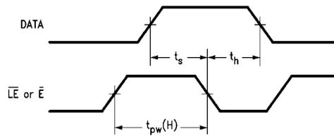
FIGURE 4. Setup, Hold and Pulse Width Times
