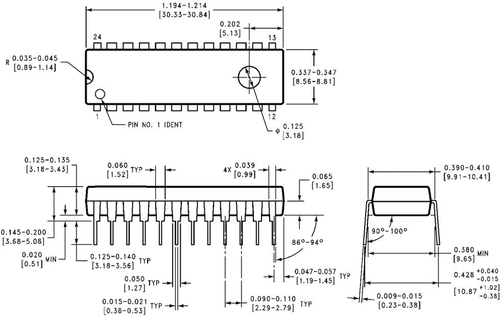
**24-Lead Plastic Dual-In-Line Package (PDIP), JEDEC MS-010, 0.400 Wide
