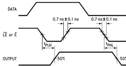
FIGURE 2. Propagation Delays
