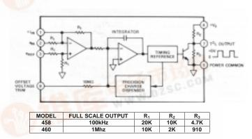
Figure 1. Block Diagram - Models 458,560
