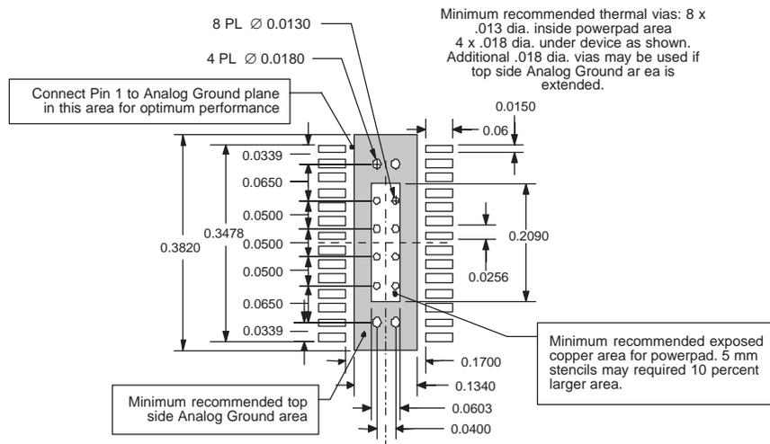
**Figure 9. Recommended Land Pattern for 28-Pin PWP PowerPAD**
