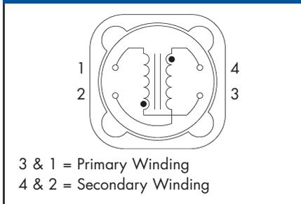
1 When connecting windings in series, inductance will be 4 times the nominal figure shown.
