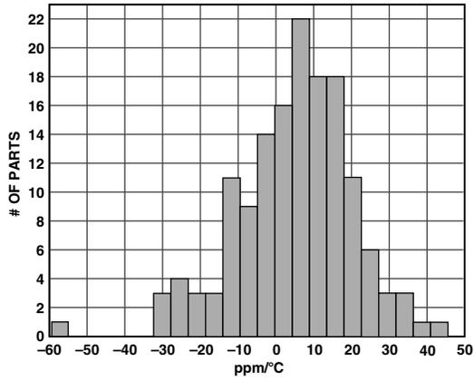
TPC 1. Typical Output Voltage Temperature Drift Distribution
