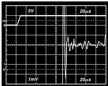
Figure 12c. Turn-On Settling
