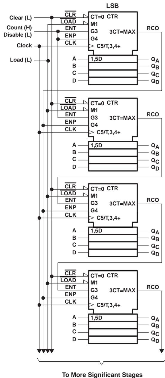
$$f_{max} = 1/(\text{CLK to RCO } t_{PLH}) + (\text{ENP } t_{su})$$
