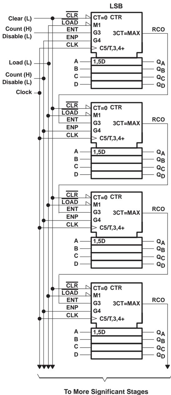
$$f_{max} = 1/(\text{CLK to RCO } t_{PLH}) + (\text{ENT to RCO } t_{PLH}) (N - 2) + (\text{ENT } t_{su})$$
