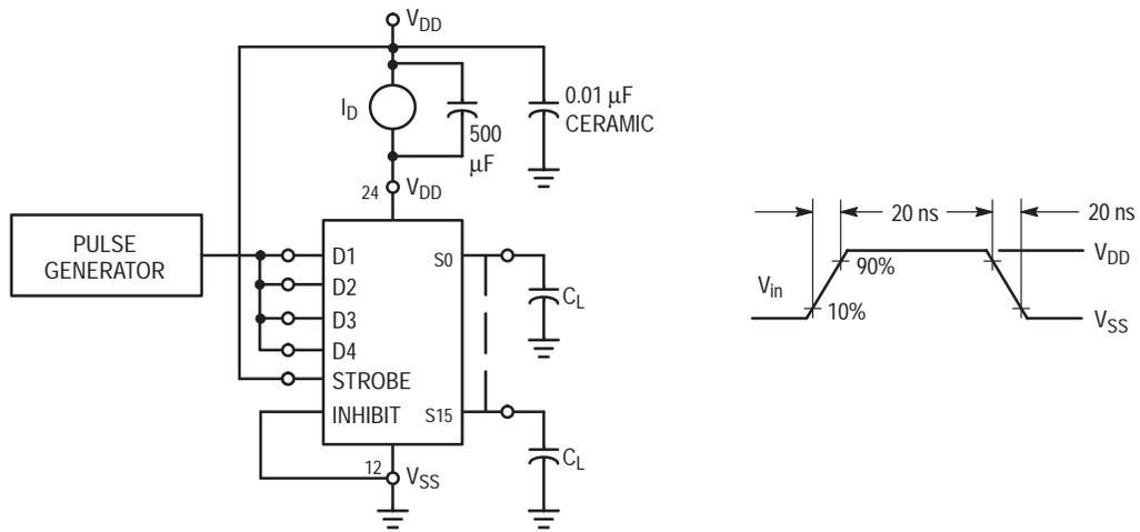
Figure 2. Dynamic Power Dissipation Test Circuit and Waveform
