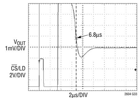
$V_{CC} = 5V$ ,  $V_{REF} = 4.096V$
