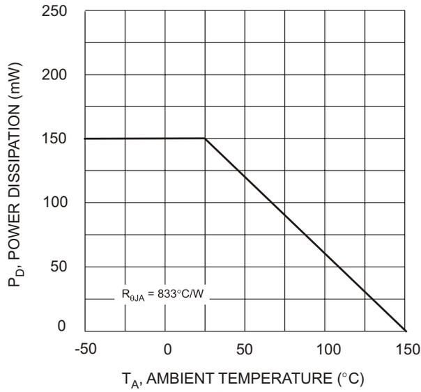
Fig. 1 Derating Curve
