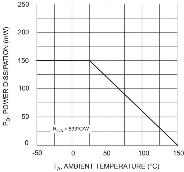
Fig. 1 Derating Curve
