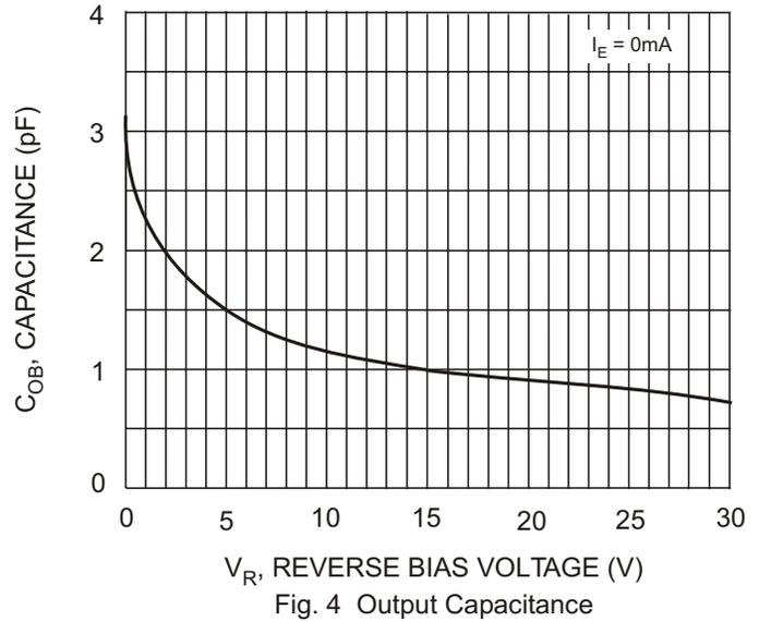
Fig. 4 Output Capacitance
