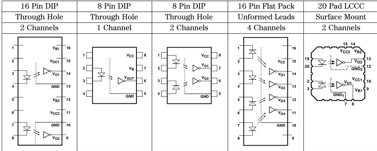
**Note:** 8 pin DIP and flat pack devices have common  $V_{CC}$  and ground. 16 pin DIP and LCCC (leadless ceramic chip carrier) packages have isolated channels with separate  $V_{CC}$  and ground connections.
