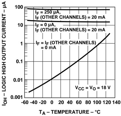
Figure 4. Logic High Output Current vs. Temperature.
