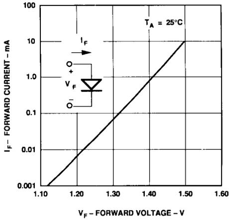
Figure 1. Input Diode Forward Current vs. Forward Voltage.
