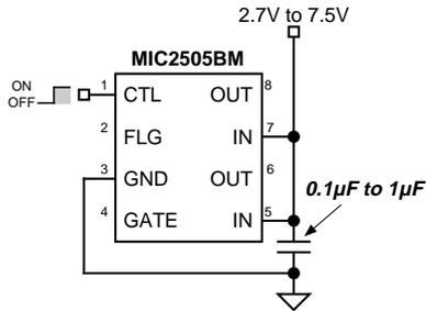
Figure 1. Supply Bypassing
