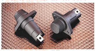
Panel mount fuseholders are available for supplementary or Class CC branch circuit protection. Class CC fuses have a rejection feature on one end cap which mates with the rejection feature of Littelfuse Class CC fuse blocks and fuseholders to prevent the installation of fuses with lower voltage ratings or interrupting ratings. Watertight version must be front panel mounted.
