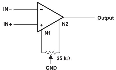
Figure 2. Input Offset Voltage Null Circuit
