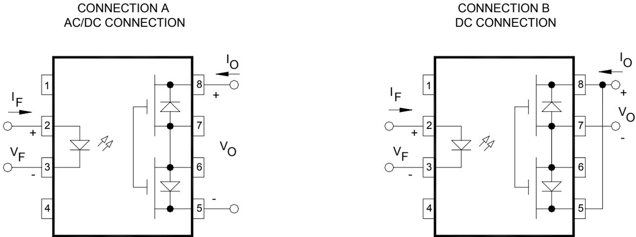
Figure 1 - Terminal Connections
