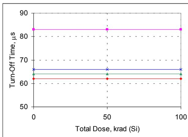
Figure 11. Turn-Off Time vs Total Dose at  $V_{out} = 28\text{ V}$ ,
