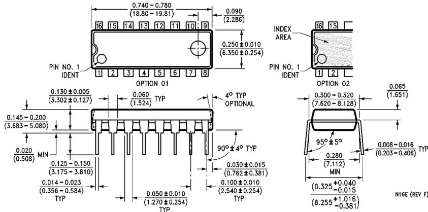
**16-Lead Molded Dual-In-Line Package (N)**
