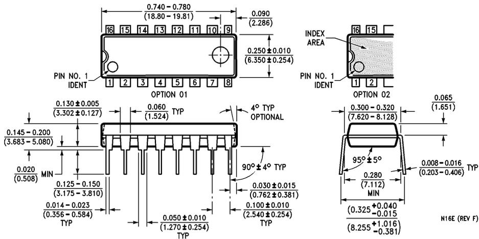
**16-Lead (0.300" Wide) Molded Dual-In-Line Package (P)**
