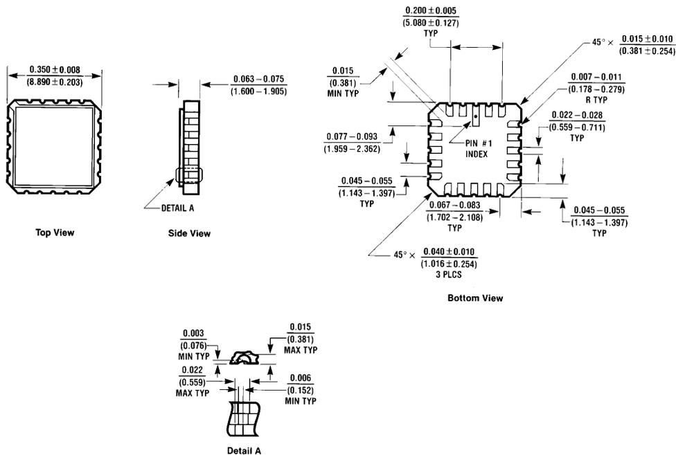
**20-Lead Ceramic Leadless Chip Carrier (L)
