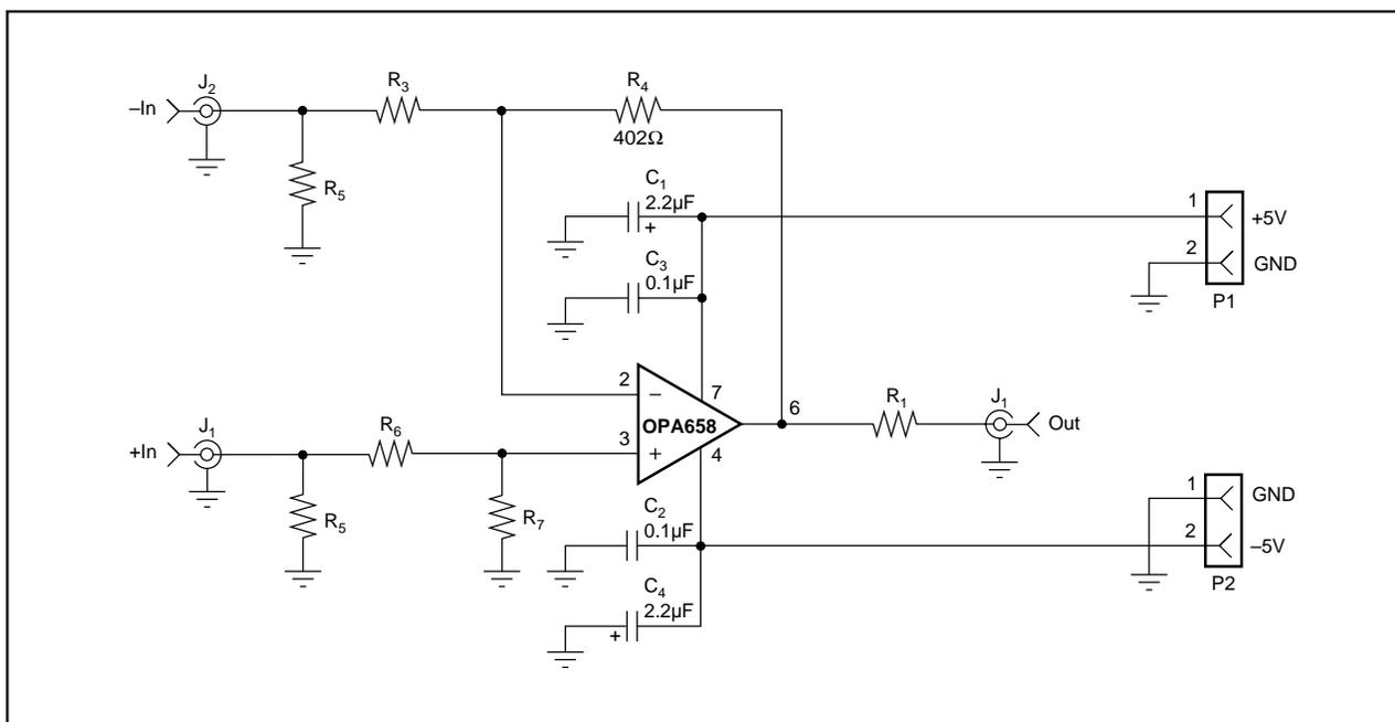
FIGURE 9. Layout Detail For DEM-OPA65xP Demonstration Board.
