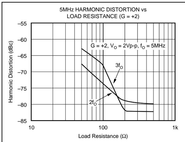
FIGURE 6. 5MHz Harmonic Distortion vs Load Resistance.
