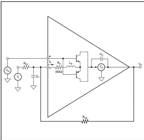
FIGURE 1. Equivalent Circuit.
