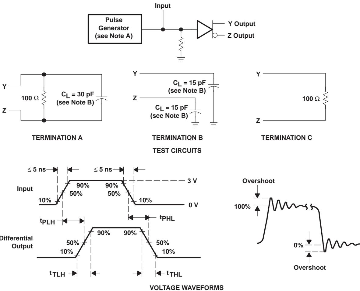
NOTES: A. The pulse generator has the following characteristics:  $Z_O = 50 \Omega$ ,  $t_W = 25 \text{ ns}$ ,  $\text{PRR} \leq 10 \text{ MHz}$ .
