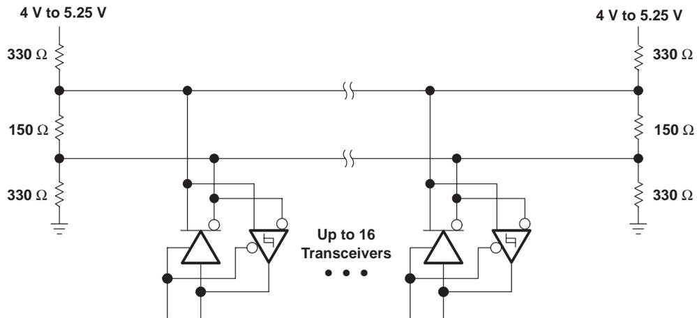
Figure 17. Typical Differential SCSI Application Circuit
