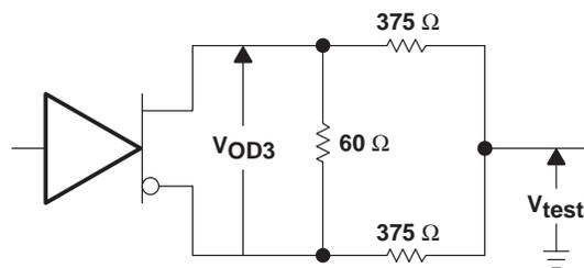
Figure 2. Driver  $V_{OD3}$
