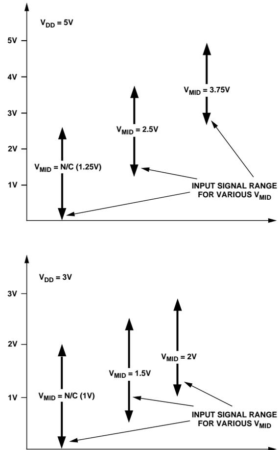
Figure 7. Analog Input Span Variation with  $V_{MID}$
