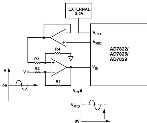
Figure 10. Accommodating Bipolar Signals Using Internal  $V_{MID}$
