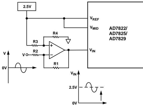
Figure 9. Accommodating Bipolar Signals Using External  $V_{MID}$
