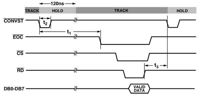
Figure 4. Track-and-Hold Timing
