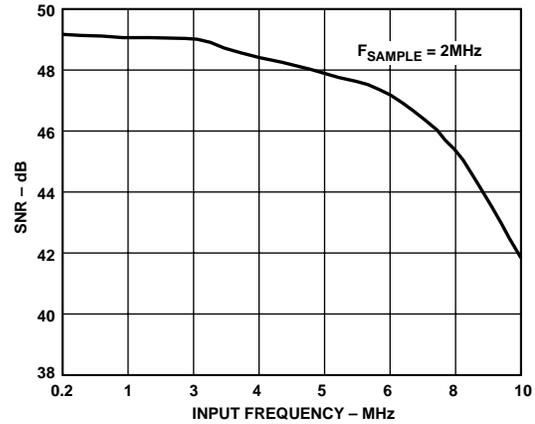
Figure 14. SNR vs. Input Frequency on the AD7825
