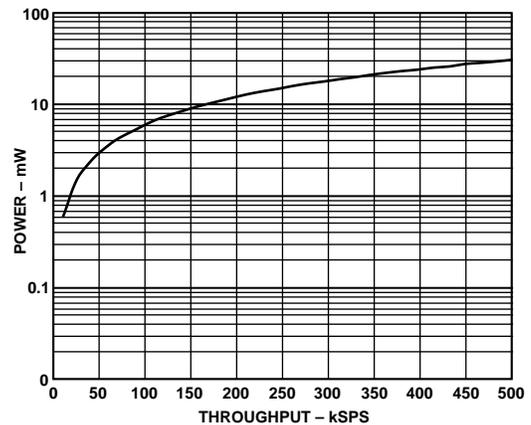
Figure 18. AD7822/AD7825/AD7829 Power vs. Throughput
