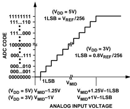
Figure 6. Transfer Characteristic
