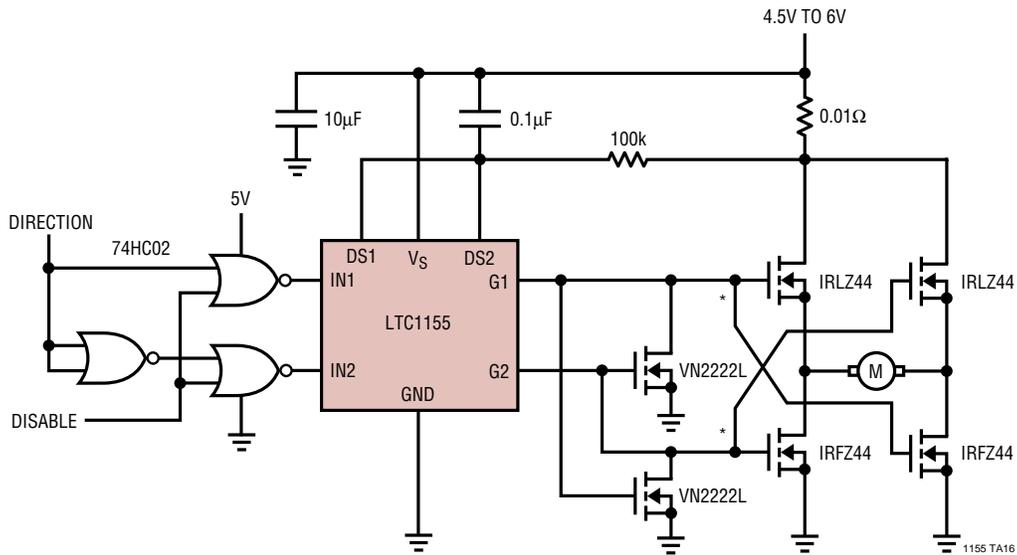
DC Motor Speed and Torque Control for Cordless Tools and Appliances
