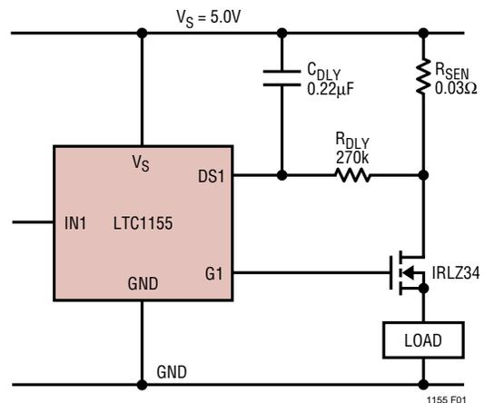
Figure 1. Adding an RC Delay
