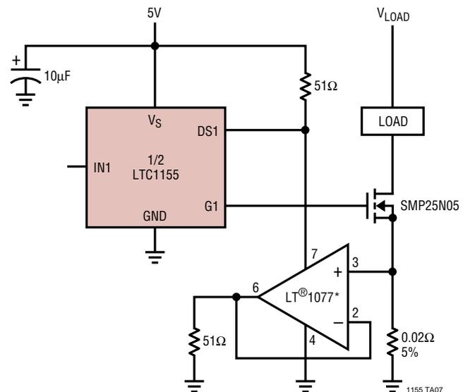
\*DO NOT SUBSTITUTE. MUST BE A PRECISION, SINGLE SUPPLY, MICROPOWER OP AMP ( $I_Q < 60\mu A$ )
