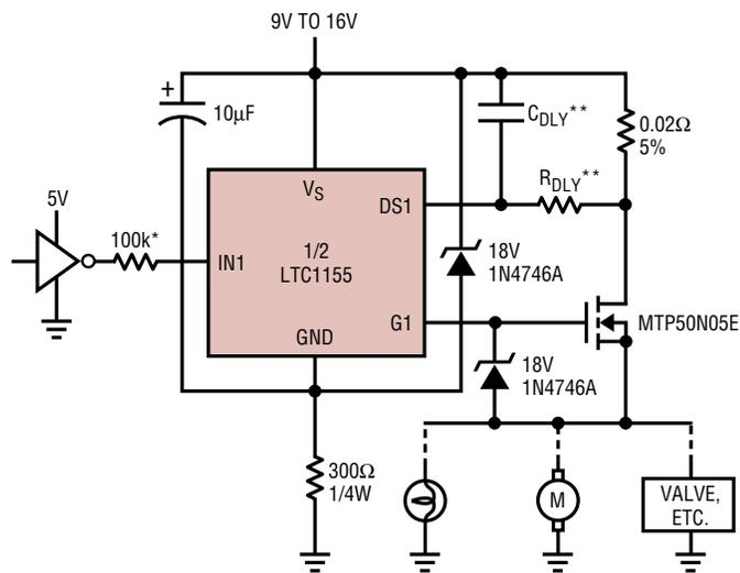
\*PROTECTS TTL/CMOS GATES DURING HIGH VOLTAGE TRANSIENT OR REVERSE BATTERY
