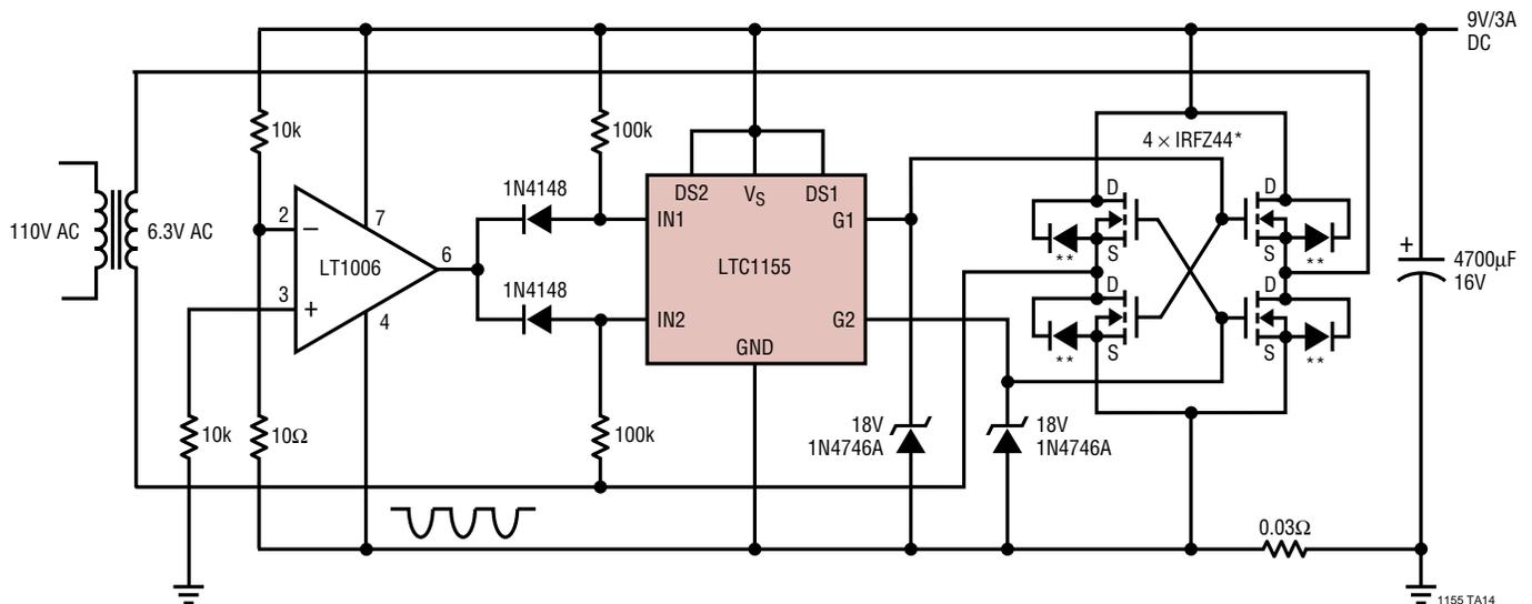
MOSFETs ARE SYNCHRONOUSLY ENHANCED WHEN RECTIFIER CURRENT EXCEEDS 300mA
