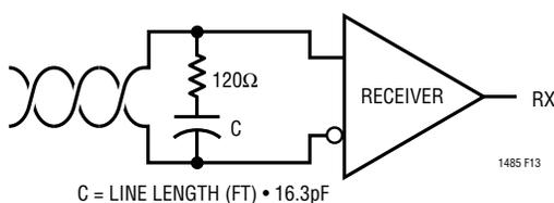
Figure 13. AC-Coupled Termination
