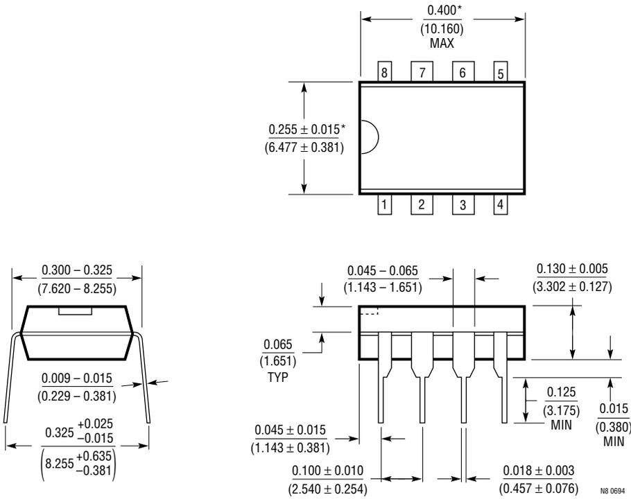
\*THESE DIMENSIONS DO NOT INCLUDE MOLD FLASH OR PROTRUSIONS.
