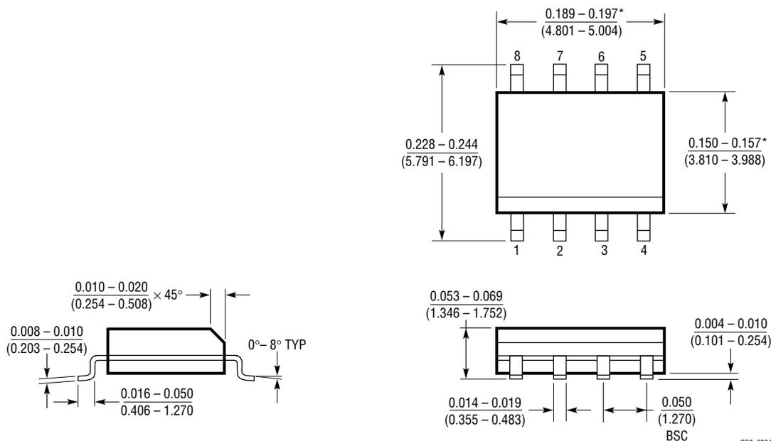
\*THESE DIMENSIONS DO NOT INCLUDE MOLD FLASH OR PROTRUSIONS.
