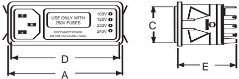
**6VM2S & 6VM4S** (IEC Connector, DPST On/Off Switch, Voltage Selector, Selectable Fuseholder)
