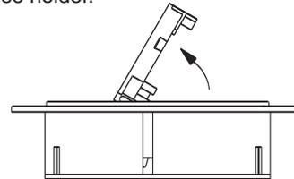
3. When the fuse holder is installed in the single fuse position, apply the screwdriver as shown and gently pry up.
