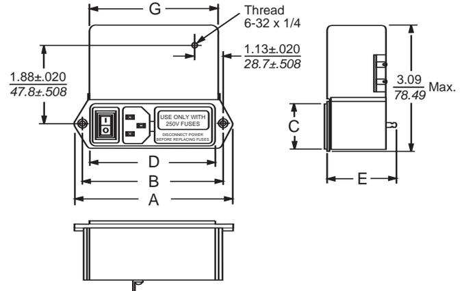
**3EXM4 & 3EZM4** (IEC Connector, Voltage Selector, Selectable Fuseholder)
