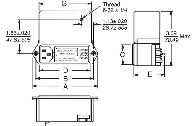
**3EXM4S & 3EZM4S** (IEC Connector, DPST On/Off Switch, Voltage Selector, Selectable Fuseholder)
