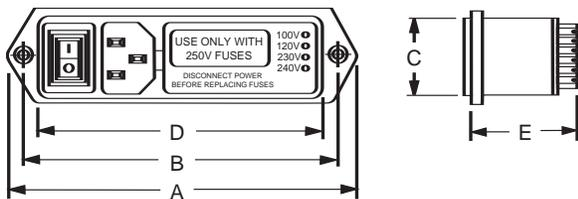
**6VM4SC** (IEC Connector, DPST On/Off Switch, Voltage Selector, Selectable Fuseholder, Snap-In)
