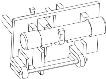
\*\*Install fuses on one side only. Do Not install both AG and Metric fuses at the same time.
