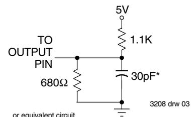
Figure 1. Output Load
