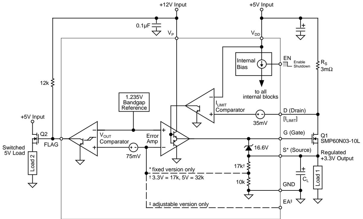
**Block Diagram with External Components
