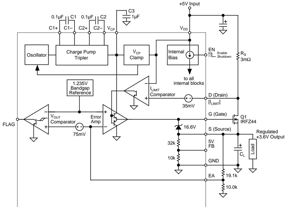
**Block Diagram with External Components
