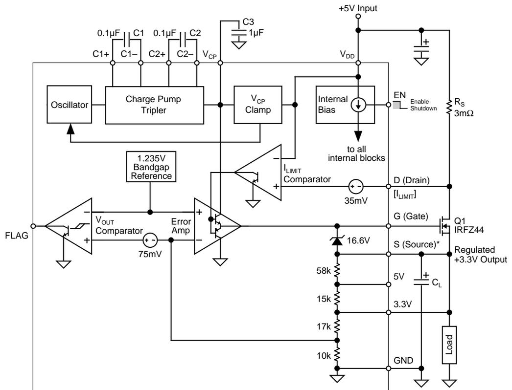
**Block Diagram with External Components
