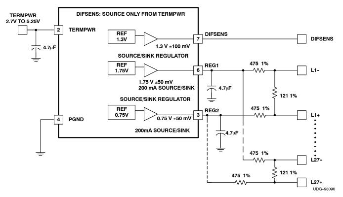
Figure 1. Low-Voltage Differential Discrete Resistor Stack
