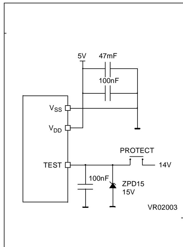
Note: ZPD15 is used for overvoltage protection
