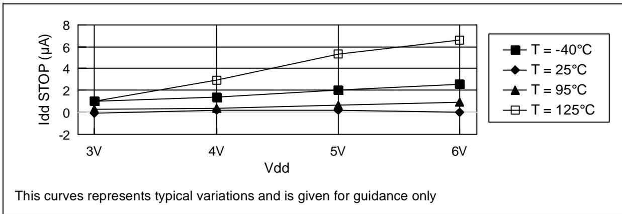
Figure 39. I<sub>DD</sub> STOP versus V<sub>DD</sub> for ROM devices
