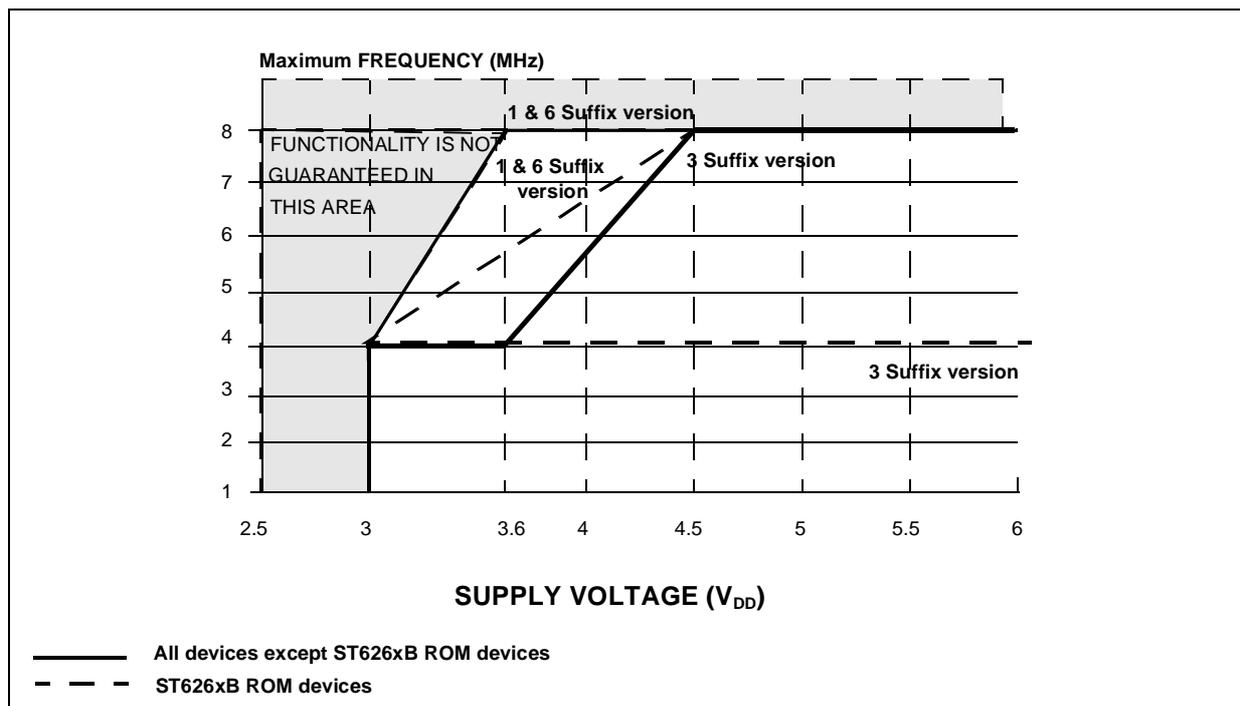
The shaded area is outside the recommended operating range; device functionality is not guaranteed under these conditions.
