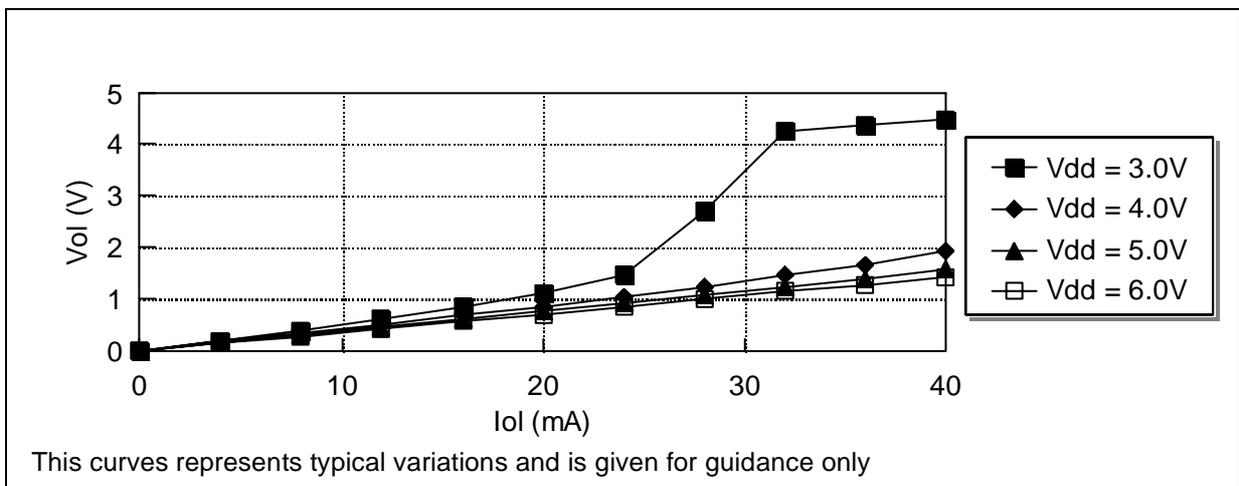
Figure 34. Vol versus Iol for High sink (30mA) I/O ports at Vdd=5V
