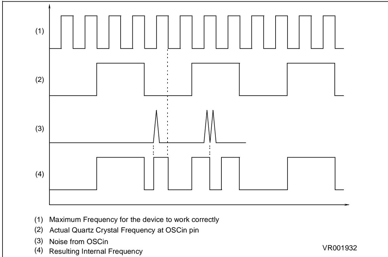
Figure 10. OSG Emergency Oscillator Principle
