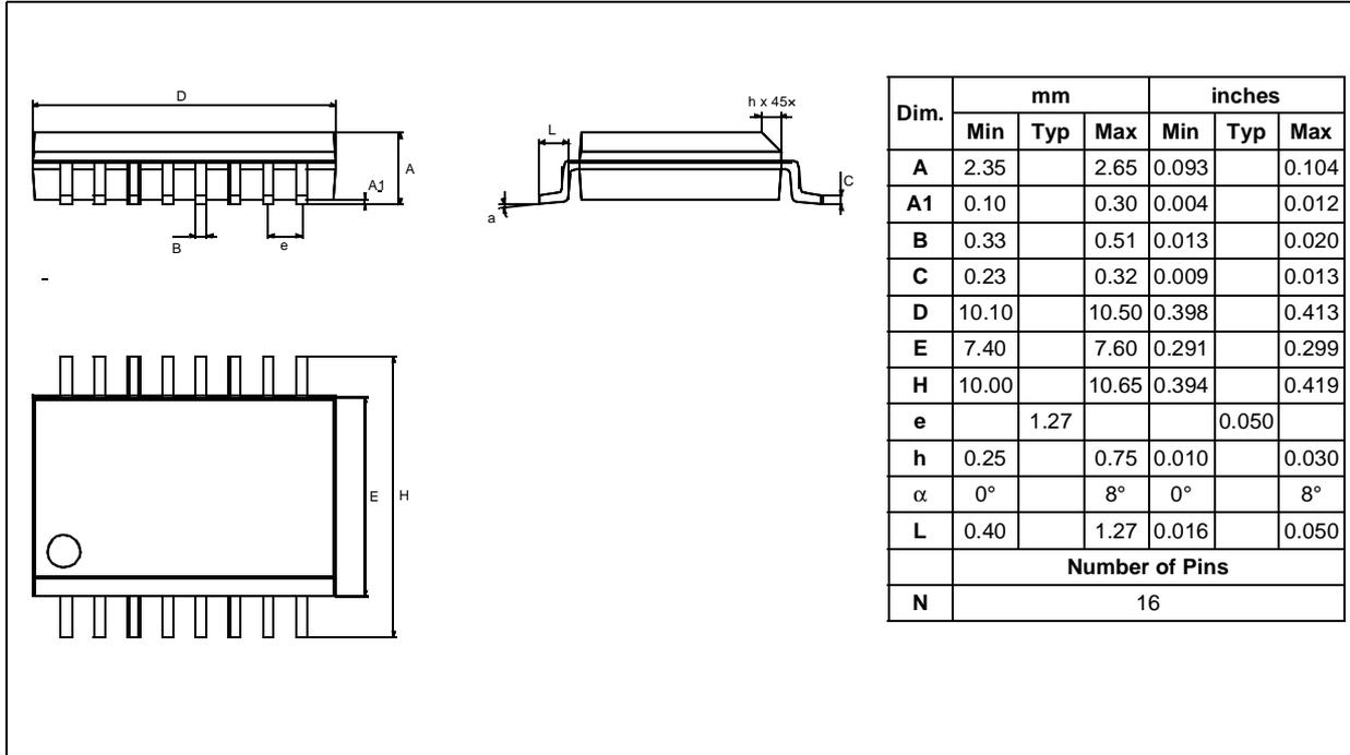
Figure 48. 16-Pin Plastic Shrink Small Outline Package
