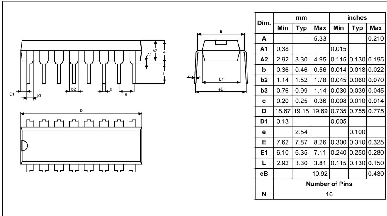
Figure 46. 16-Pin Ceramic Side-Brazed Dual In-Line Package
