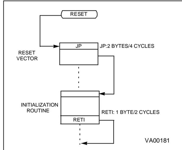
Figure 16. Reset Block Diagram
