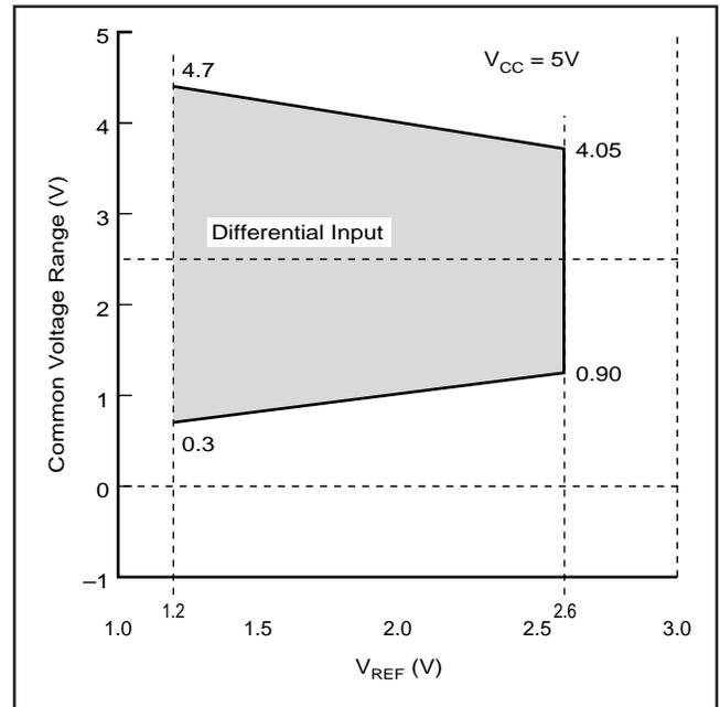
FIGURE 4. Differential Input: Common-Mode Voltage Range vs V<sub>REF</sub>.
