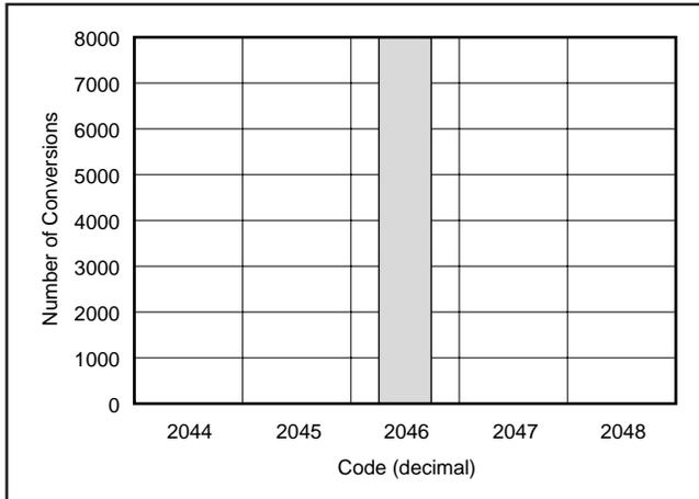
FIGURE 5. Histogram of 8,000 Conversions of a DC Input.
