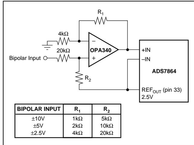
FIGURE 7. Level Shift Circuit for Bipolar Input Ranges.
