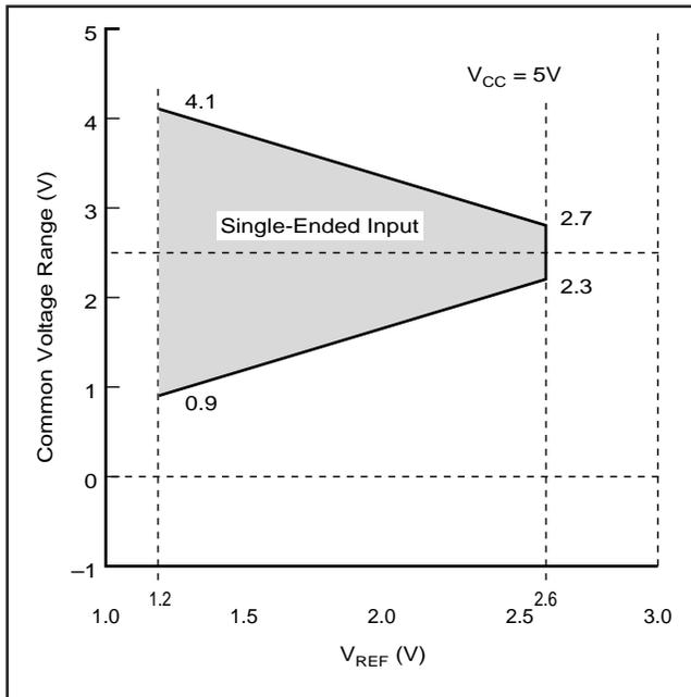
FIGURE 3. Single-Ended Input: Common-Mode Voltage Range vs V<sub>REF</sub>.
