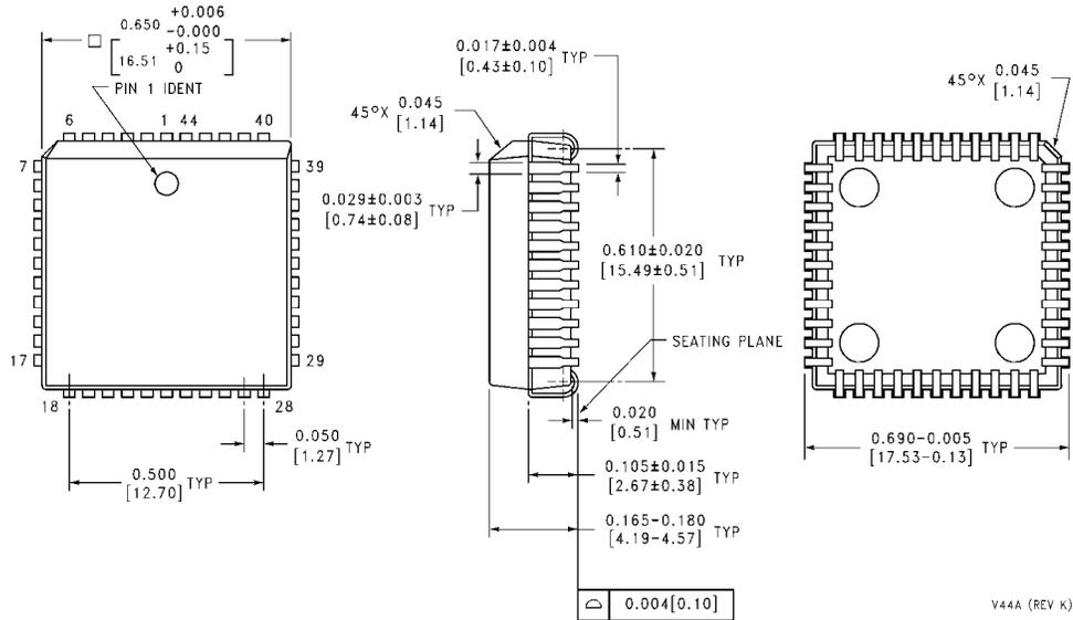
**44-Lead Plastic Lead Chip Carrier (PLCC), JEDEC MO-047, 0.650 Square
