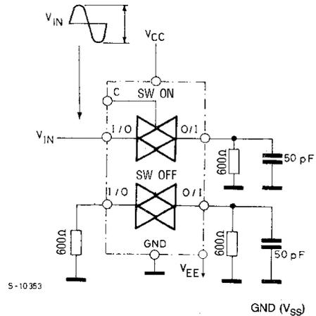
BANDWIDTH AND FEEDTHROUGH ATTENUATION
