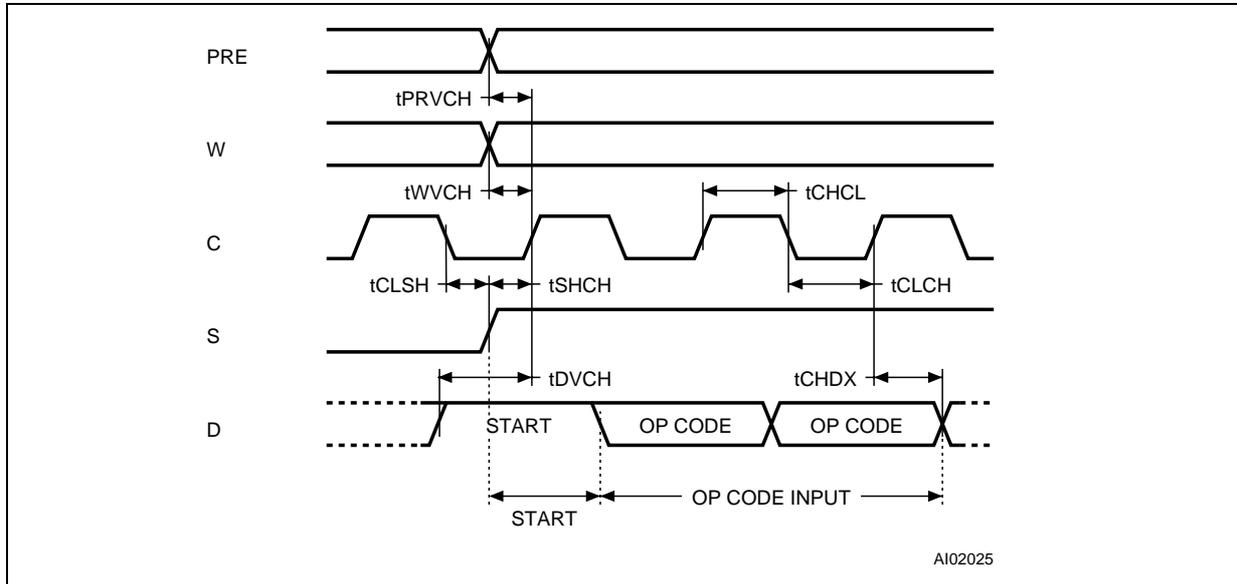
Figure 11. Synchronous Timing (Read or Write)
