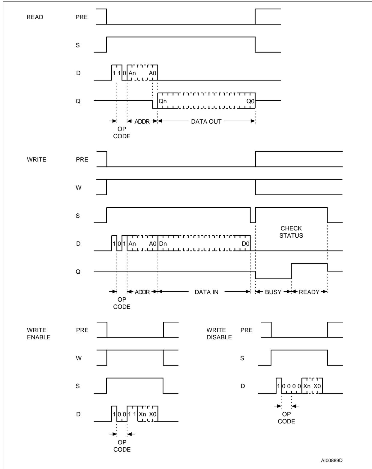
Note: For the meanings of An, Xn, Qn and Dn, see Table 2. and Table 3..
