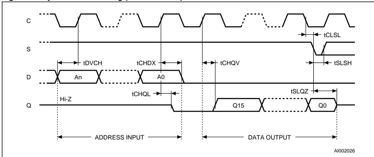
Figure 12. Synchronous Timing (Read or Write)
