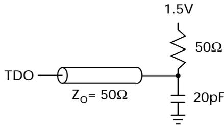
**2.5V TAP AC Output Load Equivalent**
