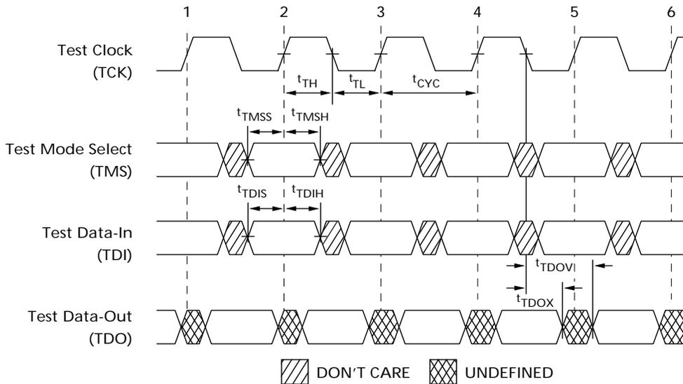
**TAP AC Switching Characteristics Over the operating Range<sup>[9, 10]</sup>**
