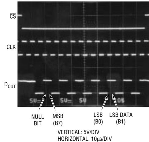
Figure 14. Scope Trace the LTC1096 “Quick Look” Circuit Showing A/D Output 10101010 (AA<sub>HEX</sub>)
