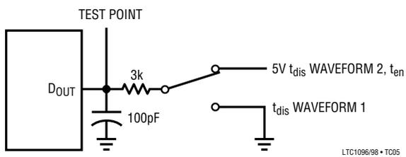
Voltage Waveforms for  $t_{dis}$
