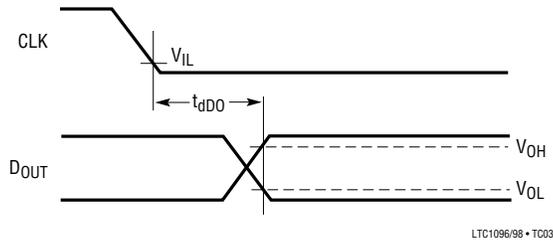
Voltage Waveforms for  $D_{OUT}$  Rise and Fall Times,  $t_r$ ,  $t_f$
