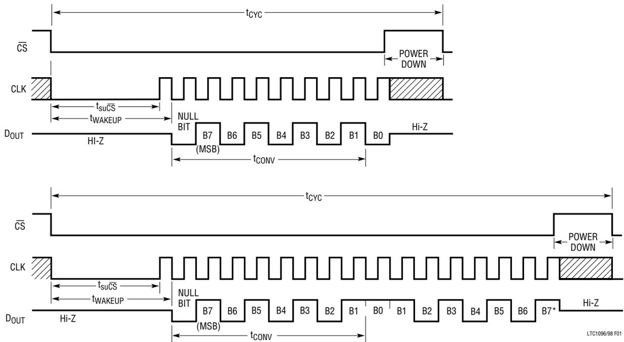
\*AFTER COMPLETING THE DATA TRANSFER, IF FURTHER CLOCKS ARE APPLIED WITH  $\overline{CS}$  LOW, THE ADC WILL OUTPUT ZEROS INDEFINITELY.
