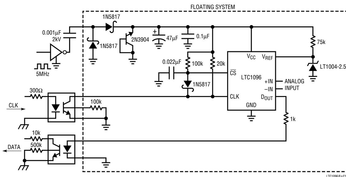
**Figure 16. Power for This Floating A/D System Is Provided by a Simple Capacitor Diode Charge Pump. The Two Optoisolators Draw No Current Between Samples, Turning On Only to Send the Clock and Receive Data**
