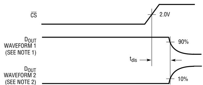
NOTE 1: WAVEFORM 1 IS FOR AN OUTPUT WITH INTERNAL CONDITIONS SUCH THAT THE OUTPUT IS HIGH UNLESS DISABLED BY THE OUTPUT CONTROL.
