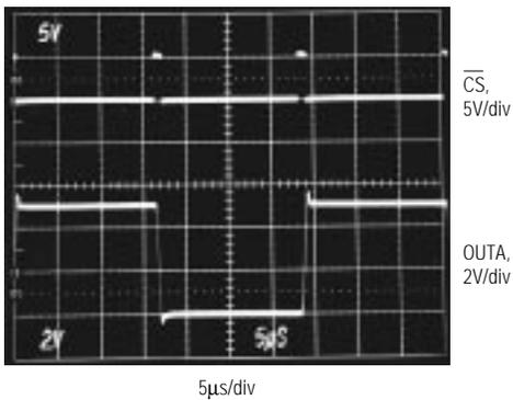
$V_{DD} = +15\text{V}$ ,  $V_{SS} = -5\text{V}$ ,  $\text{REFAB} = 5\text{V}$ ,  $C_L = 100\text{pF}$ ,  $R_L = 10\text{k}\Omega$
