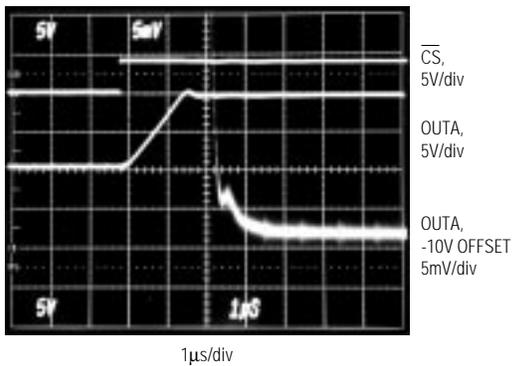
$V_{DD} = +15\text{V}$ ,  $V_{SS} = -5\text{V}$ ,  $\text{REFAB} = 10\text{V}$ ,  $C_L = 100\text{pF}$ ,  $R_L = 10\text{k}\Omega$
