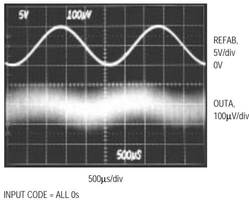
**MAX536 REFERENCE FEEDTHROUGH AT 4kHz**
