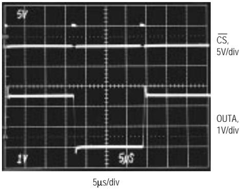
$V_{DD} = +5\text{V}$ ,  $V_{SS} = -5\text{V}$ , REFAB = 2.5V,  $C_L = 100\text{pF}$ ,  $R_L = 10\text{k}\Omega$
