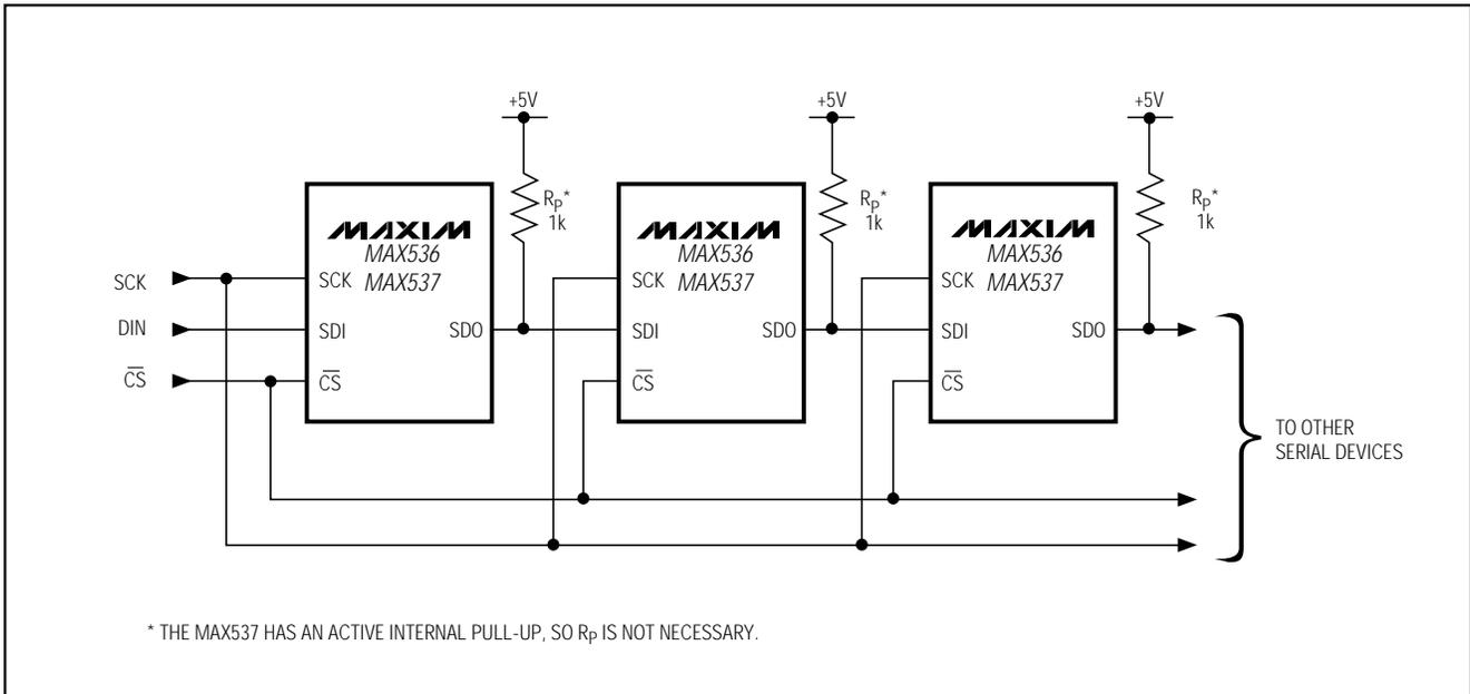
Figure 8. Daisy-Chaining MAX536/MAX537s with a 3-Wire Serial Interface
