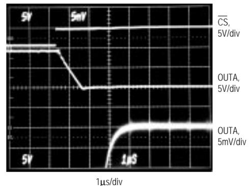
$V_{DD} = +15\text{V}$ ,  $V_{SS} = -5\text{V}$ ,  $\text{REFAB} = 10\text{V}$ ,  $C_L = 100\text{pF}$ ,  $R_L = 10\text{k}\Omega$
