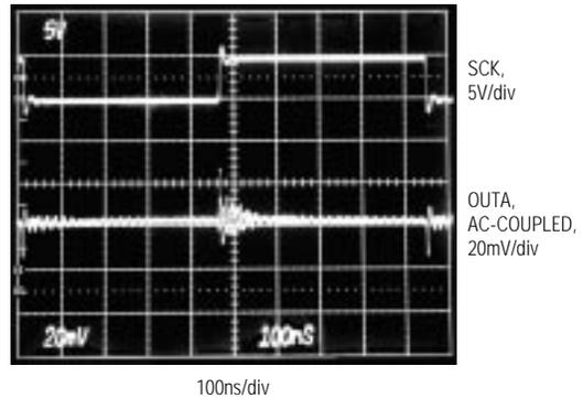
$V_{DD} = +5\text{V}$ ,  $V_{SS} = -5\text{V}$ , REFAB = 2.5V,  $\overline{\text{CS}} = \text{HIGH}$ ,
