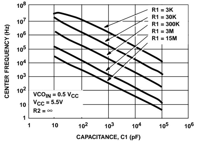
FIGURE 17. HCT7046A TYPICAL CENTER FREQUENCY vs R1, C1
