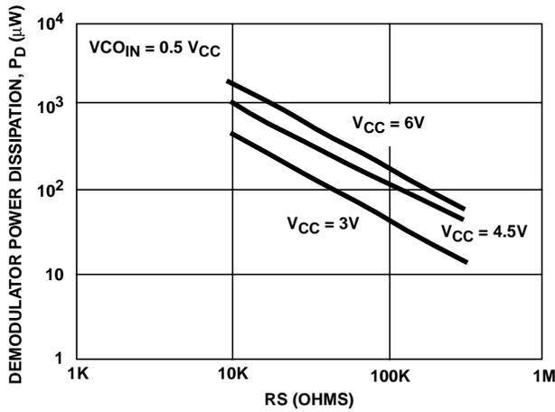
FIGURE 40. HC7046A DEMODULATOR POWER DISSIPATION vs RS (TYP)
