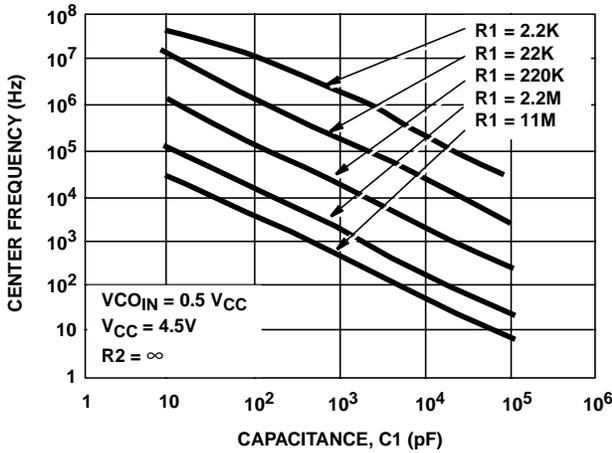
FIGURE 16. HCT7046A TYPICAL CENTER FREQUENCY vs R1, C1
