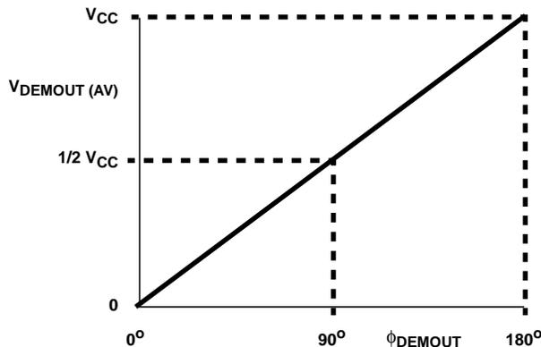
**FIGURE 2. PHASE COMPARATOR 1: AVERAGE OUTPUT VOLTAGE vs INPUT PHASE DIFFERENCE:**
