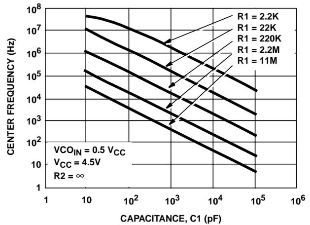
FIGURE 13. HC7046A TYPICAL CENTER FREQUENCY vs R<sub>1</sub>, C<sub>1</sub>
