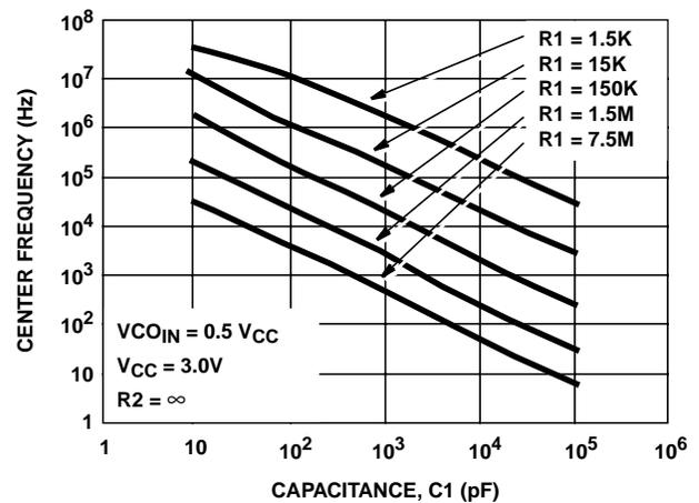
FIGURE 15. HC7046A TYPICAL CENTER FREQUENCY vs R<sub>1</sub>, C<sub>1</sub>
