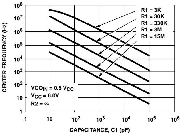
FIGURE 14. HC7046A TYPICAL CENTER FREQUENCY vs R<sub>1</sub>, C<sub>1</sub>
