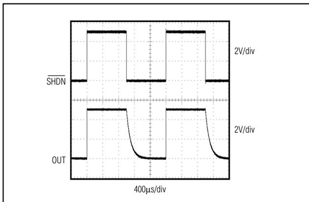
Figure 5. Shutdown Waveform
