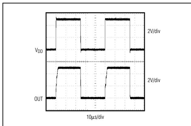
Figure 4. Power-Up/Power-Down Waveform
