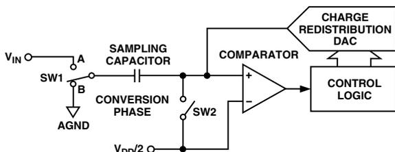
Figure 3. ADC Conversion Phase
