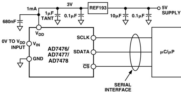
Figure 6. REF193 as Power Supply to AD7476/AD7477/AD7478
