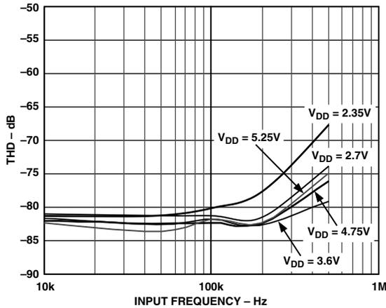
Figure 9. THD vs. Analog Input Frequency,  $f_s = 993$  kSPS
