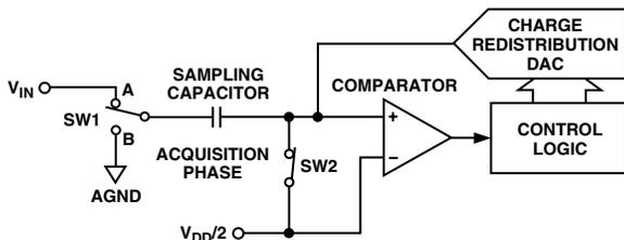
Figure 2. ADC Acquisition Phase
