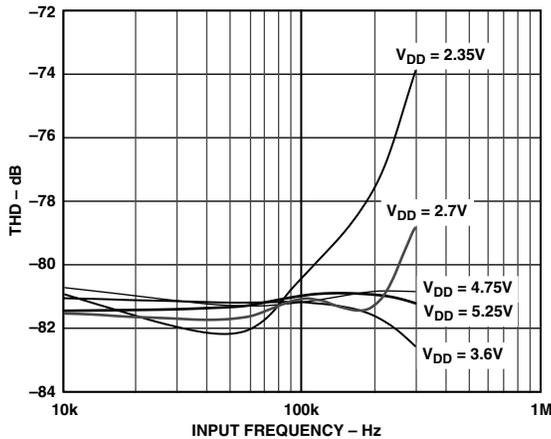
Figure 10. THD vs. Analog Input Frequency,  $f_s = 605$  kSPS
