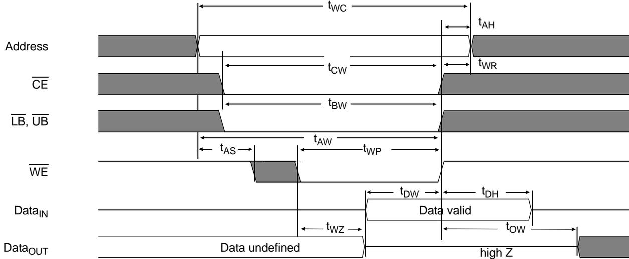
**Write waveform 2 ( $\overline{\text{CE}}$  controlled)<sup>10,11</sup>**
